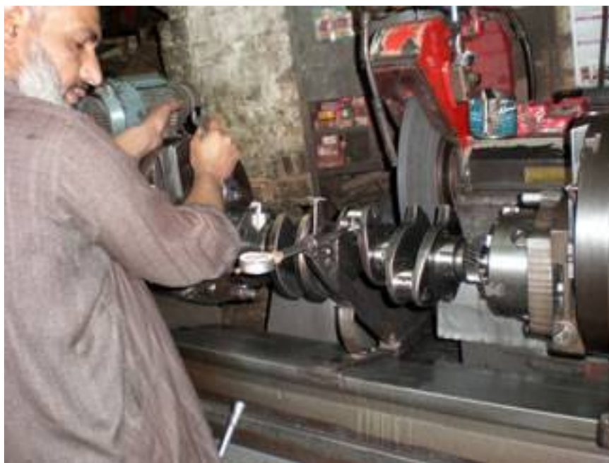
Machining on a tractor crankshaft in a medium size set-up in Peshawar
